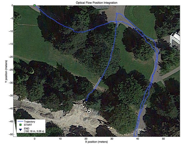
Fig. 9. Integrated metric output of the PX4FLOW sensor with Google Map overlay for a flight along a promenade.
