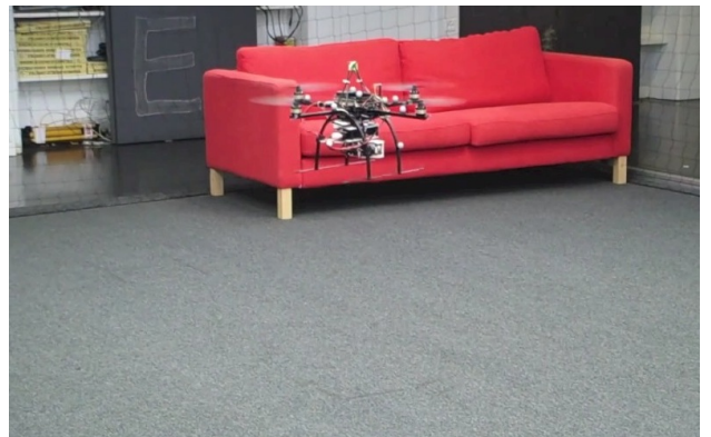
Fig. 5. PIXHAWK Cheetah hovering in an indoor lab environment with PX4FLOW faced downwards
