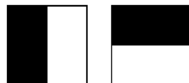
Fig. 9. Haar wavelet filters to compute the responses in x (left) and y direction (right). The dark parts have the weight -1 and the light parts +1 .
