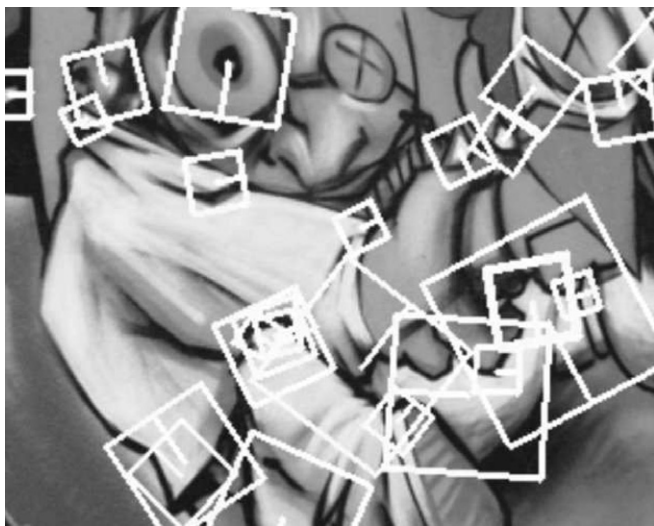
Fig. 11. Detail of the Graffiti scene showing the size of the oriented descriptor window at different scales.
