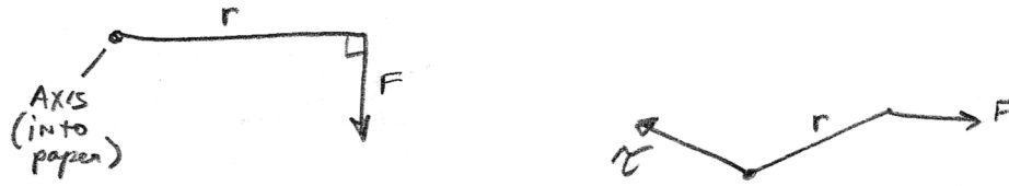
Figure 3.1: An applied force F generates a torque if it acts through a point having a radius, r from the axis of rotation. Left: force is applied perpendicular to the moment arm. Right: force is applied in a general direction. (see text).
